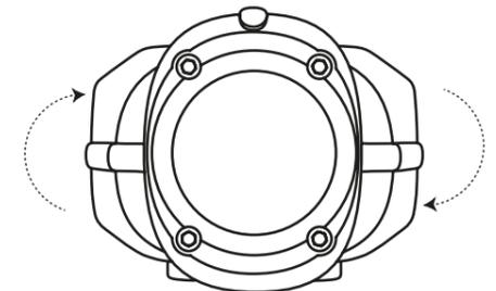
**!** The camera lens cannot be rotated through 360° – it can only be rotated through a range of 300°. At either end of this range, there is a hard stop. Do not force the camera rotation past this point, as you risk damaging the components. If excess resistance is experienced, double-check that you have not reached the camera rotation stop.
