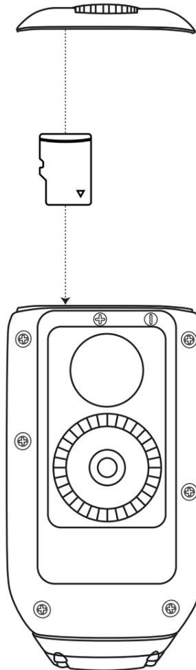
**!** Ensure that the camera is powered off when inserting and removing a memory card. The card and the data may be damaged if inserted or removed while the camera is turned on.
